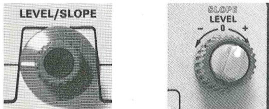
Fig. 4. Two methods of handling the TRIGGER LEVEL and SLOPE function. Both functions are accomplished with one control shown at left. Concentric controls at right accomplish both functions and occupy about the same front-panel space.
